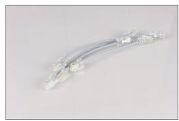
the plug in their insulation). The CAN bus signal is quite resistant to interference from external sources, however, it is not recommended to lead the bus cables parallel to the power supply cables (it is necessary to keep a distance between them). The CAN bus cable should be fixed in one section (connection is not recommended) and terminated on both sides with RJ45 plugs.
